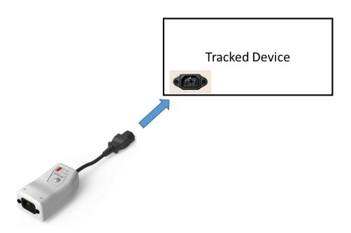
1. Insert the Tag's C13 cable into the C14 connector on the device to be tracked.
