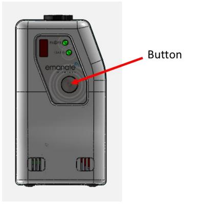
**Note** If the Status LED does not flash after pressing the button, the battery may have been run down. In that case, you should first charge up the tag by plugging it into an AC outlet for 2 hours.
