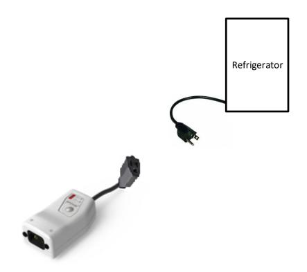
1. Insert the assets male NEMA5-15 into the Tag's NEMA5-15 female connector
